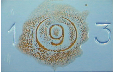
Magnetic powder visualization
