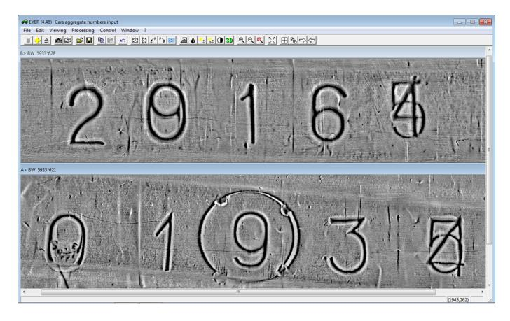
The software is intended for non-destructive examination of metal surface for authenticity verification and detection of VIN, firearms and ammunition identification number falsification, restoration of original identification numbers, verification of vehicle and firearms related documents.
